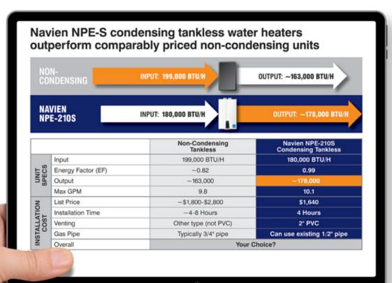
The NPE-S condensing tankless water heaters are so efficient that they outperform much larger capacity non-condensing competitors.
